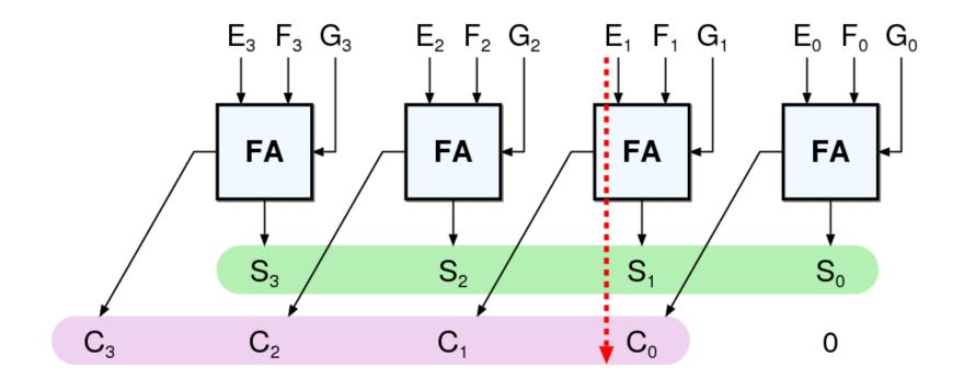
Reduces three numbers to two with a single gate delay
