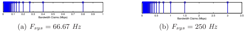
Fig. 12. Achievable bandwidth claims by traffic shapers in the packet-pair technique. A spike at value X indicates that bandwidth X can be achieved.
